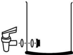
tighten it firmly. You will not need any tools to tighten the nut. The rubber rings will hold the tap in place preventing leakage.
